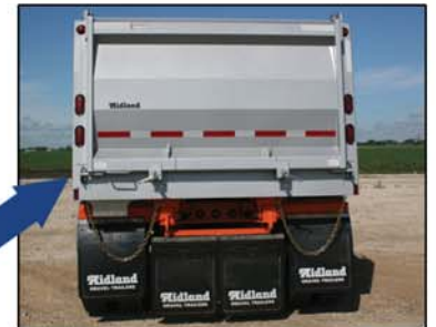
Rear Gate with Sealed Gate Option and High Visibility Lighting
