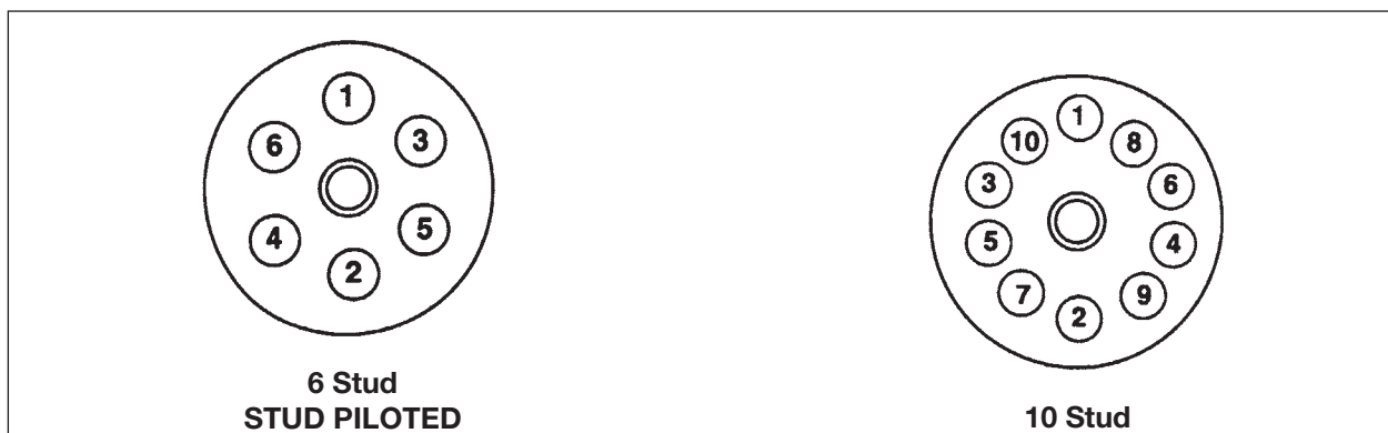
Fig. 44 NUT TORQUE SEQUENCE
