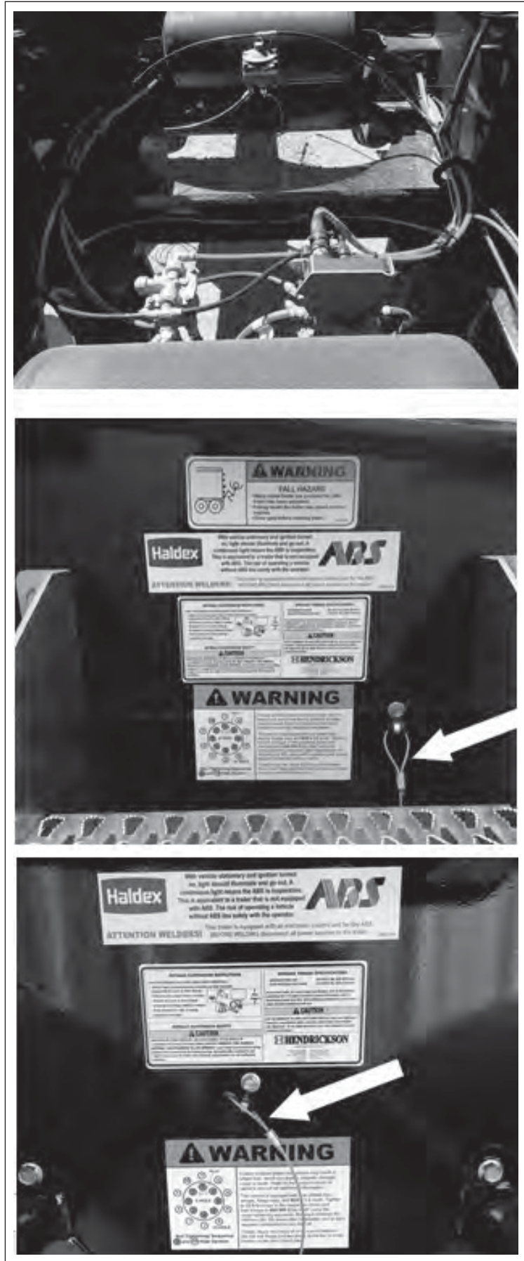
Fig. 13 DRAIN CABLES (TYPICAL)
