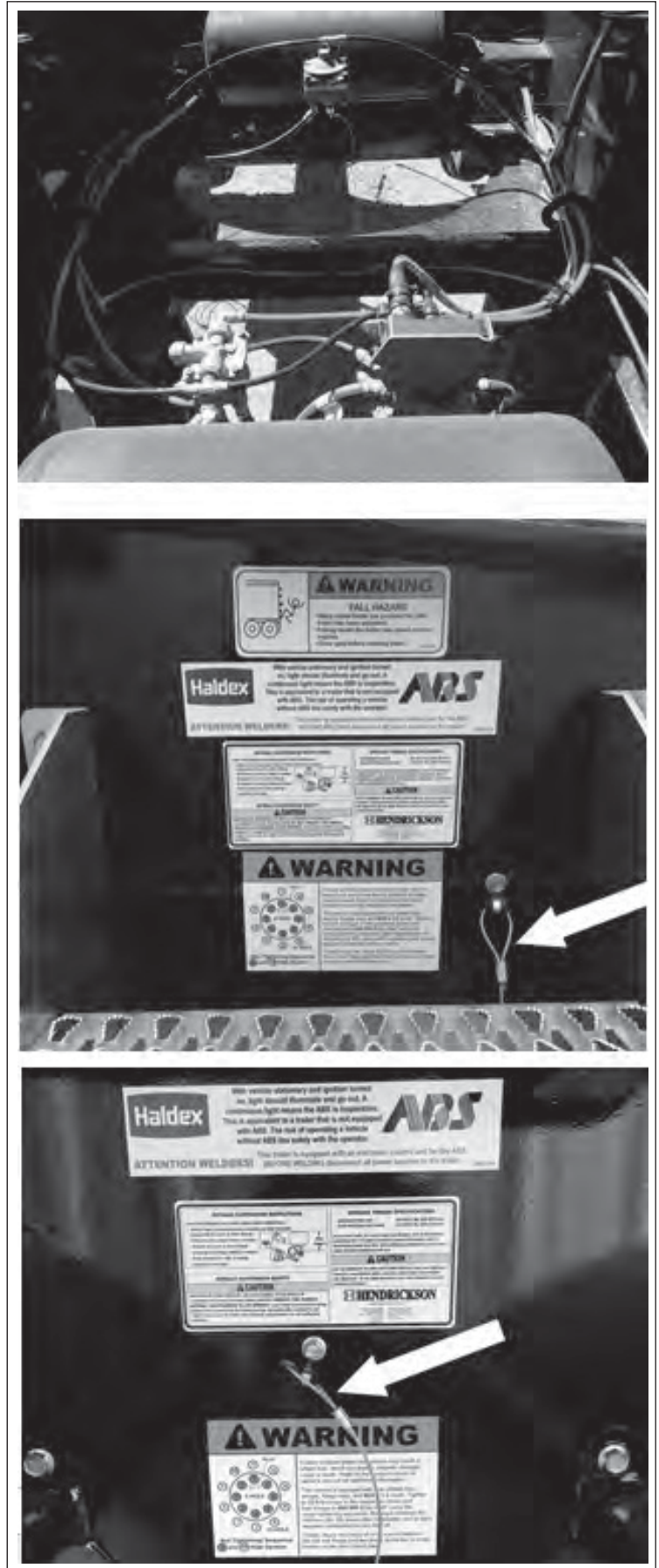
Fig. 2 DRAIN VALVE CABLE
