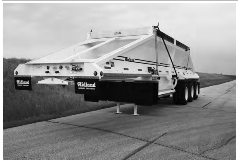
Fig. 46 CLAM TRAILER (TYPICAL)
