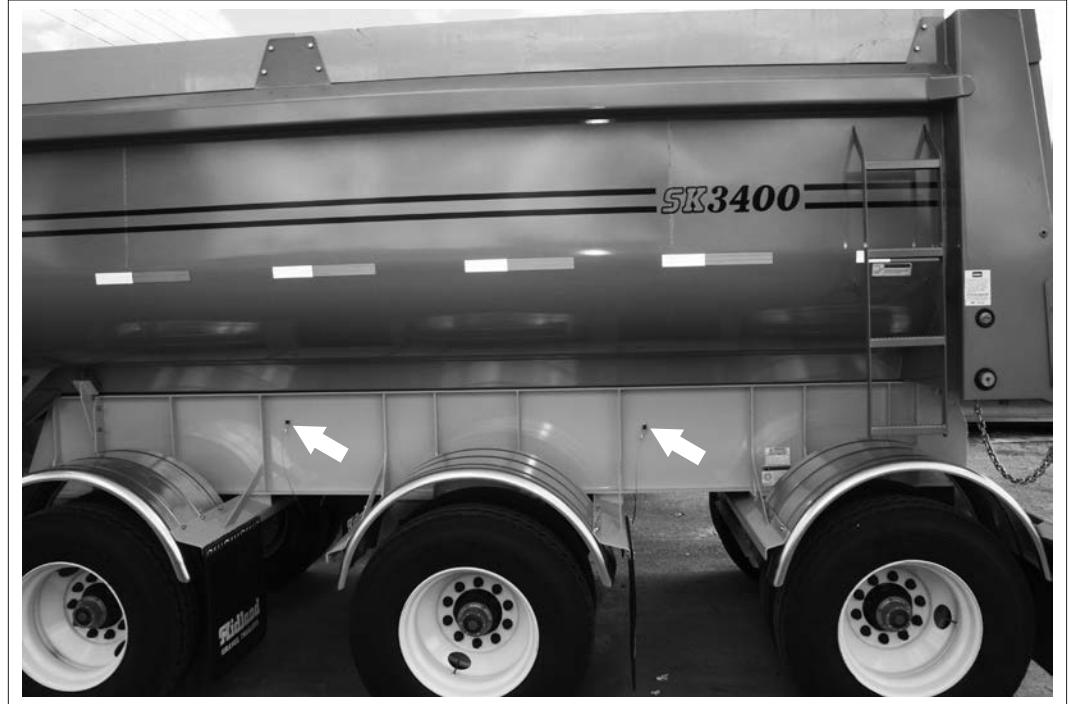
Fig. 25 DRAIN CABLES (TYPICAL)
