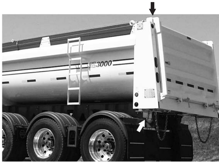
Full Frame (Pony Pup, Wagon and Full Frame models have 2 pivot point locations)
